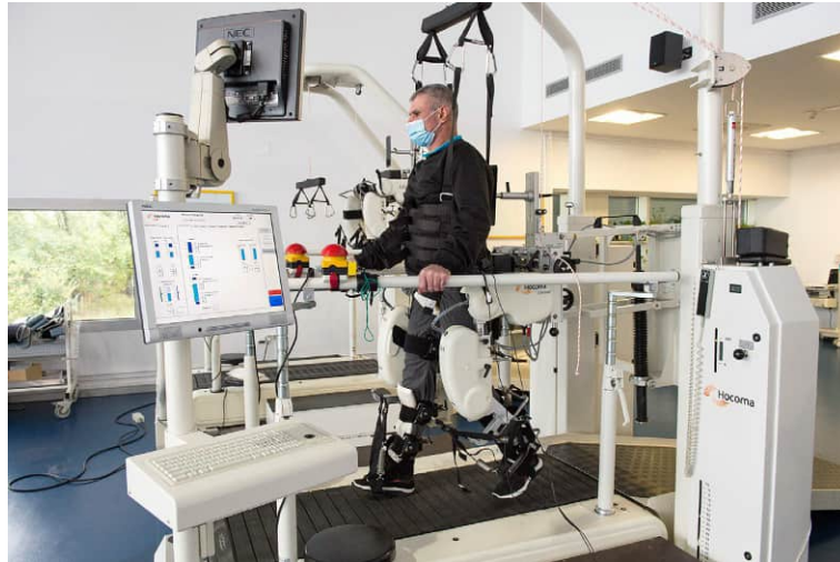
FIG. 3 Lokomat. Lokomat system with a spinal cord-injured patient.
